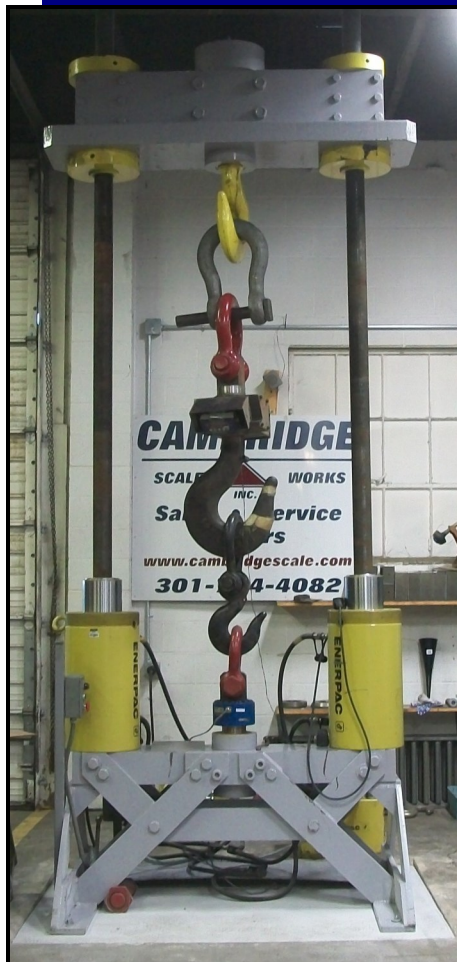
100,000 lb Crane Scale Calibration Press
