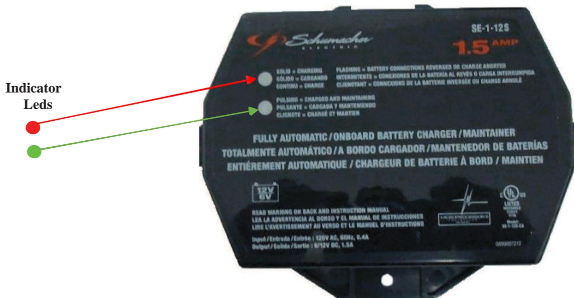
2. Connect the battery charger unit to a 110VAC outlet. The red charge indicator LED will turn on solid to indicate that the charging unit is fast charging the battery.
