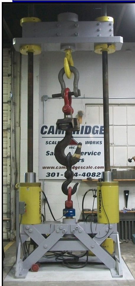
100,000 lb Crane Scale Calibration Press
