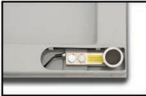
The Cambridge Scale Works, Inc. Model 660 "PLUS" utilizes four load cells with adjustable leveling feet pocketed in the scale frame for durability and accuracy.
